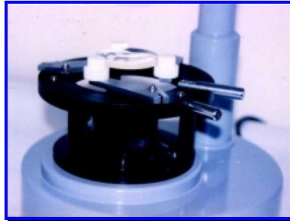
The centring checking system displays deviation error for lenses that transmit in the visual spectrum. This single axis system is a neat self-contained unit displaying the error on built-in analogue meter, an ideal quality assurance instrument that can be used in both the standards room and the shop-floor.
