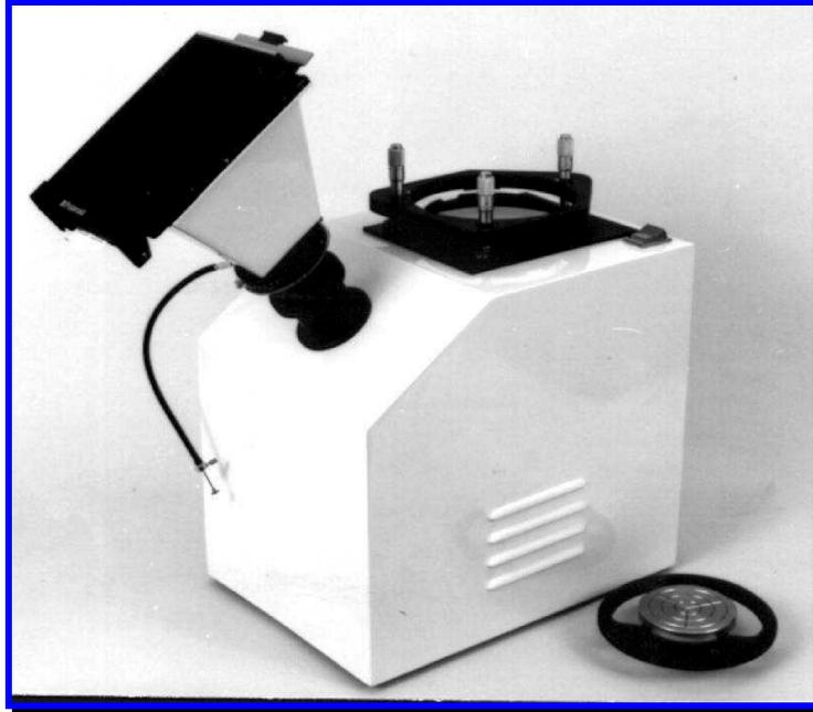
These interferometers can be built to a variety of specifications affording standard accuracy of up to 1/10 wavelength flatness over 80% of the operation reference flat diameter thus offering economy with purpose need.
